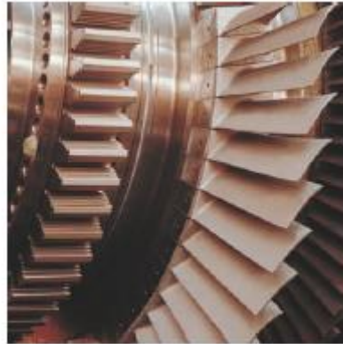
Figure (32) Turbine blades attached to the turbine shaft.
