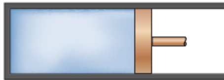
Figure (22) Quasi-equilibrium expansion and compression of a gas (reversible processes)
