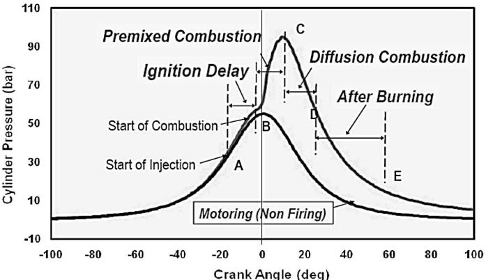
**1**. Ignition delay (a-b) : period is counted from the start of injection to towards the actual burning. The liquid fuel atomizes into small drops. The fuel vaporizes and mixes with the high-temperature high-pressure air.
